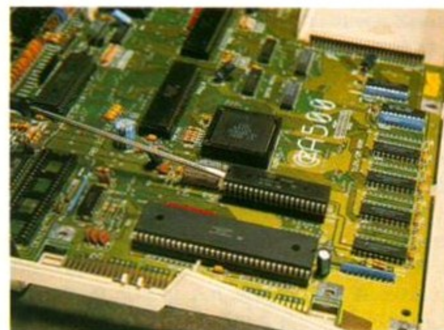
The Kickstart 2.04 ROM chip is necessary in order to use Workbench 2. Luckily it's also the easiest chip to physically get at – you can get your screwdriver low enough to apply plenty of leverage.
